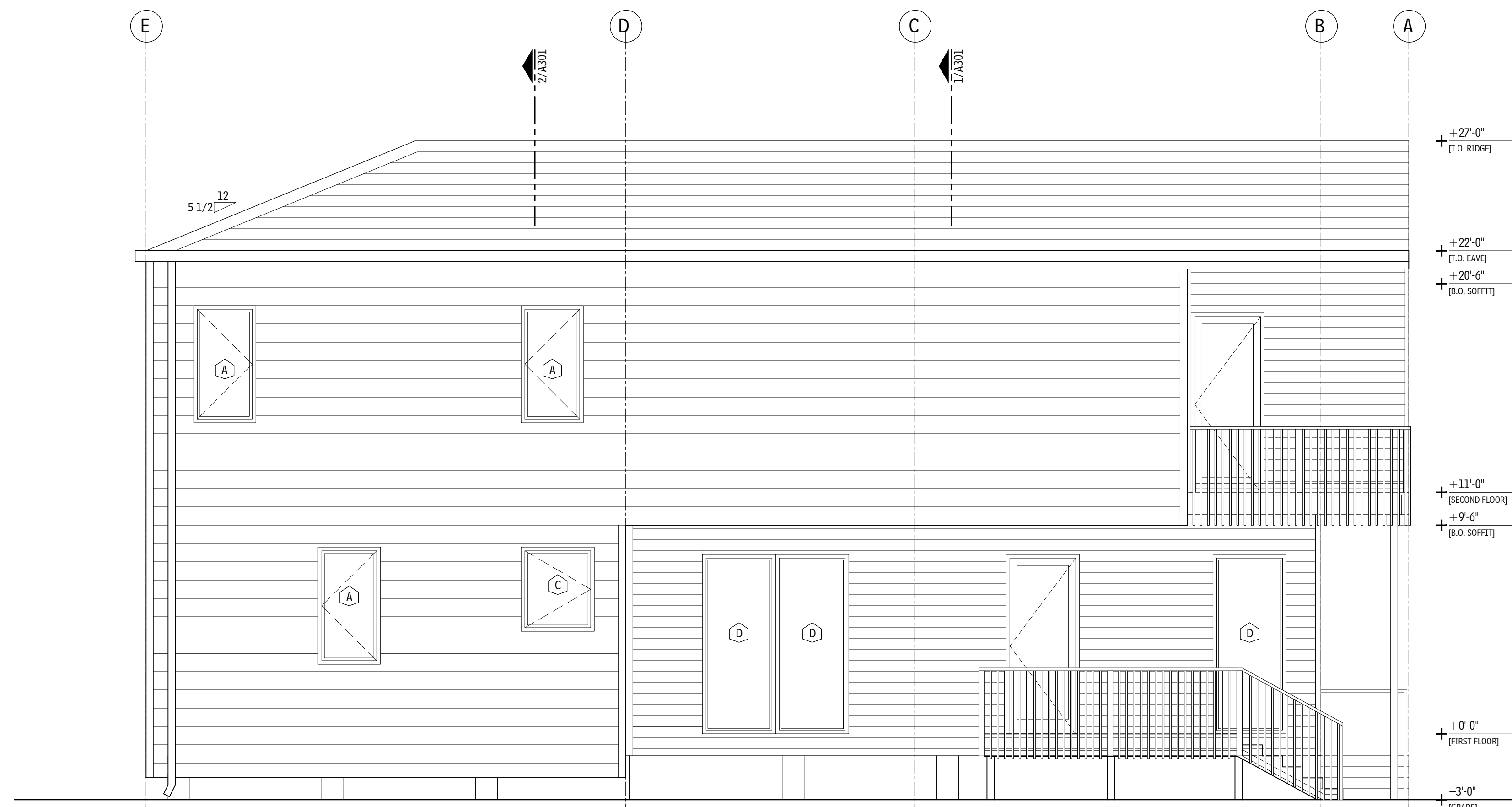
4 WEST BUILDING ELEVATION SCALE: 1/4" = 1'-0"
